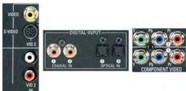
Figure 18 – Video 2 AV, Digital Audio and Component Video Inputs
