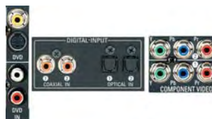
Figure 20 – DVD AV, Digital Audio and Component Video Inputs
